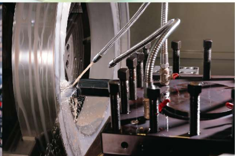
CNC车床执行精密加工 Die mold cutting operation on CNC lathe machine
